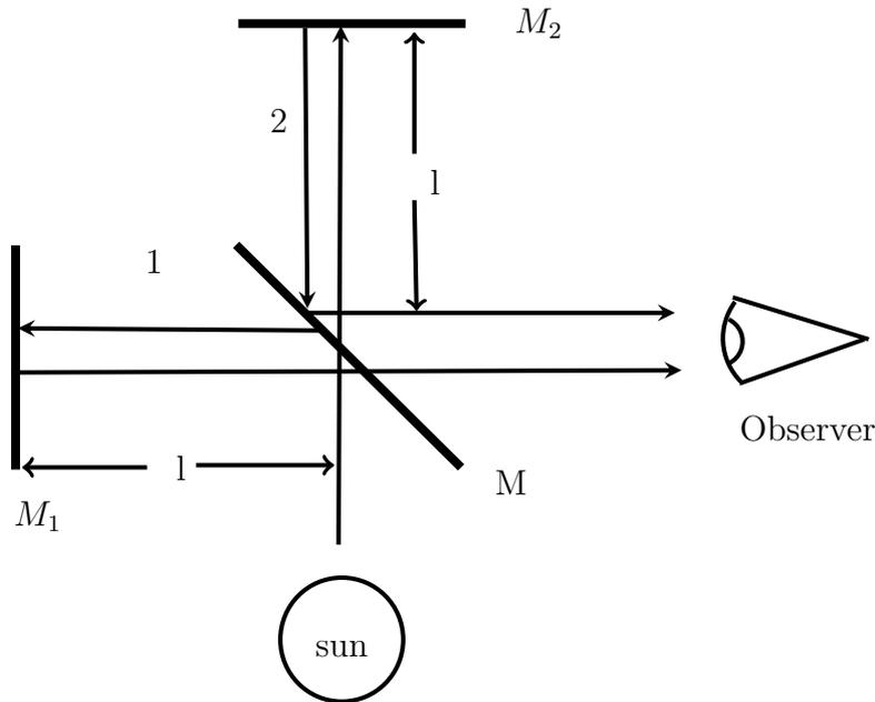
Figure 1: Schematic diagram of the Michelson interferometer.
